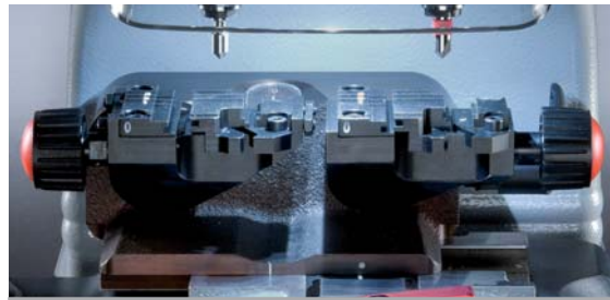
Tilting clamp (0° +/- 45°) with four seats of key positioning
